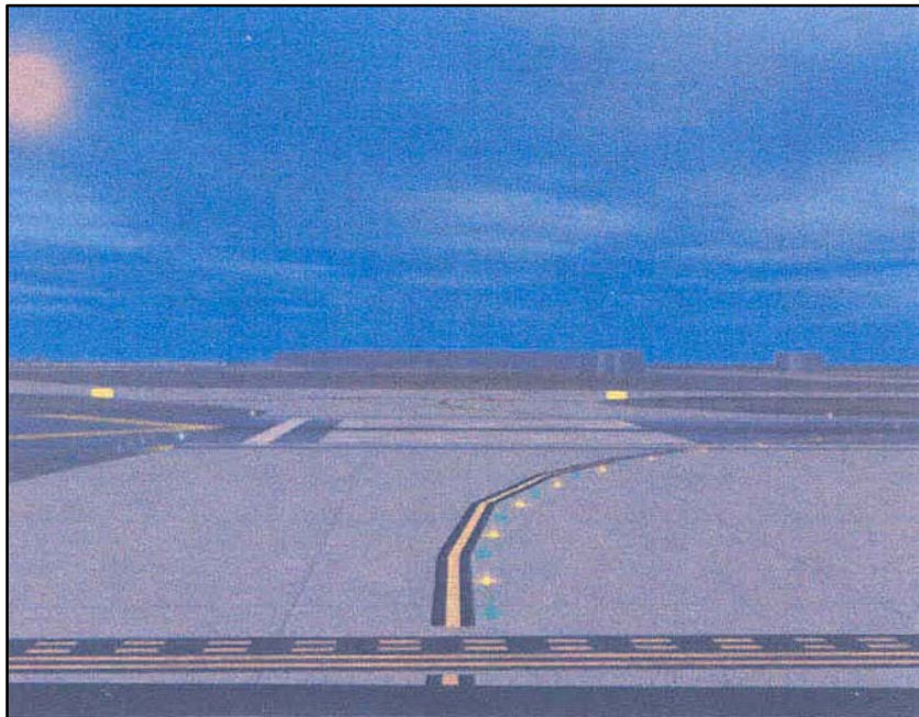
FIG 2-1-12 Taxiway Lead-On Light Configuration
